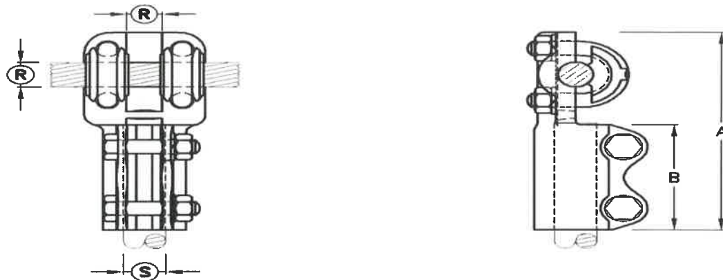
Drawing: 10 Horizontal to vertical stud clamp for stranded to solid Conductor
